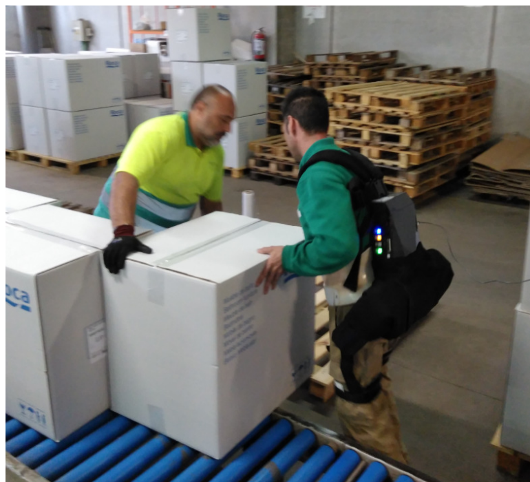
Figure 6 – Early tests with an available prototype of exoskeleton at the palletization area in ROYO.
